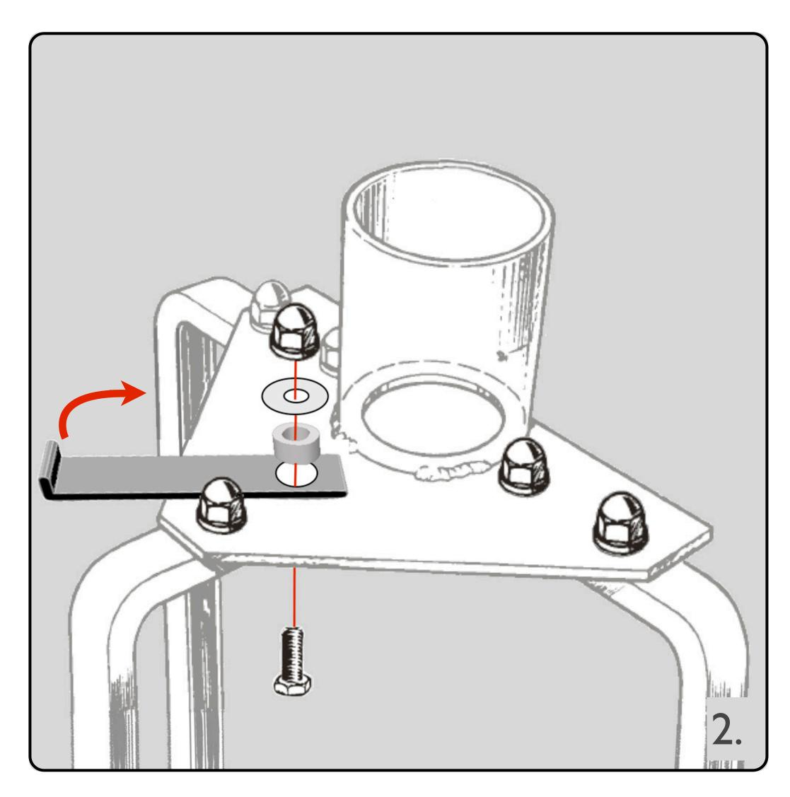
2. Attach the socket plate to the top of the L-brackets using the acorn nuts, bolts and lock washers. On one of the inside bolts, attach the propane cover support hook. The support hook uses a nylon bushing and a flat washer and will be able to swivel and support the propane cover when changing the propane tank.
